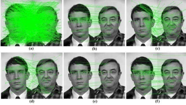
Fig. 4. Correspondence points found between the image pairs of the same view (Frontal view); (a) Potential correspondence points obtained using Lowe's method [23]; (b) Ground truth found manually; (c), (d) and (e) RANSAC method with different models and (f) Our method.
