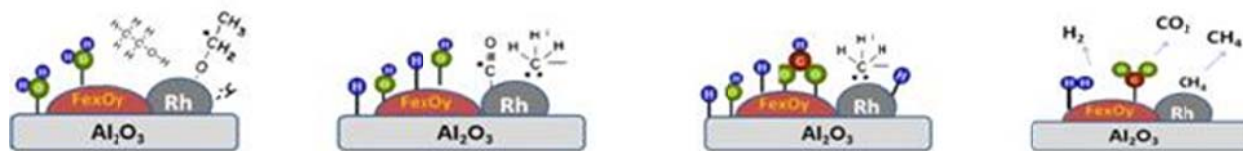
Scheme 1 Proposed ESR mechanism over Rh-Fe/Ca-Al 2 O 3 catalyst
