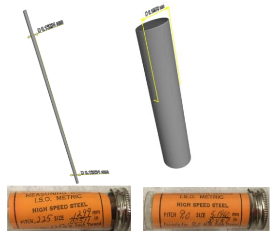
Figure 13. Examples to show XCT images of 2 standard cylinders measured diameters of \phi 132.3\ \mu\text{m} and \phi 5199.8\ \mu\text{m} by the proposed XCT.
