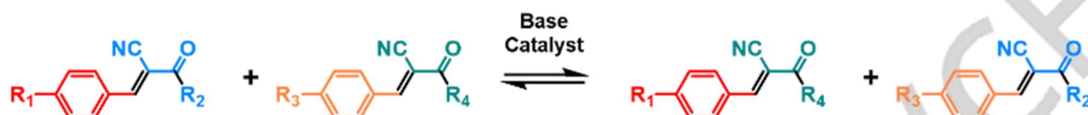
Figure 8. Schematic representation of conventional C=C metathesis and Knoevenagel adduct enabled C=C metathesis reactions.
