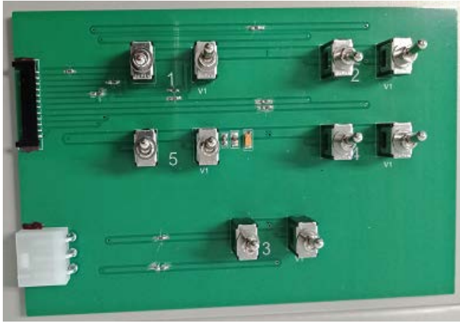
Fig. 5. Manual RF switching control board.
