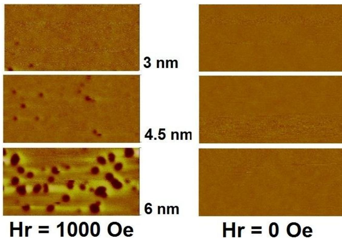
Figure 4: MFM images of the samples with different SFI layer thicknesses, measured at a reverse field ( $H_r$ ) of 1000 Oe and 0 Oe.
