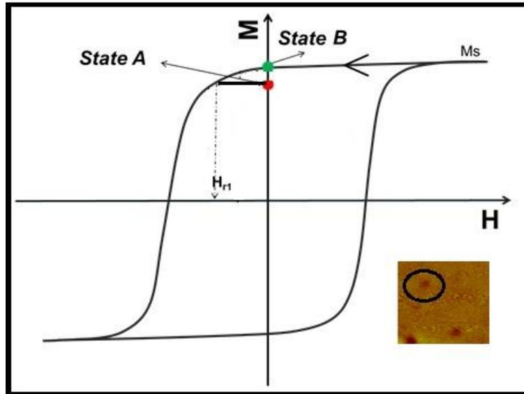
Figure 2: (a) Schematic illustration of the magnetic states at which MFM measurements were carried out. State A represents measurement at remanence after the application of a reversal field  $H_{r1}$ , which is a fraction of  $H_n$ . State B represents measurement at remanence after saturation (Inset) Typical MFM image of a media sample with reversed captured at the State A. The circled regions and similar (uncircled) dots are the reversed regions most probably due to stacking faults.
