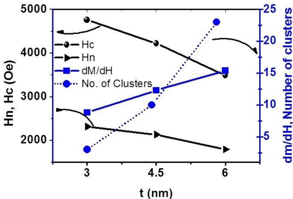
Figure 5: Effect of SFI layer thickness on the coercivity, nucleation field,  $dM/dH$  and number of clusters observed in MFM.
