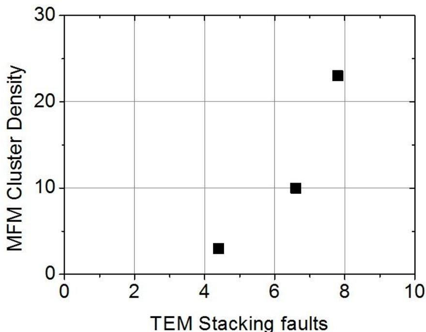
Figure 7. Correlation between the MFM cluster density and the number of stacking faults measured using cross-section TEM
