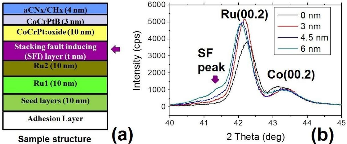
Figure1: (a) A sketch of the media layer structure with approximate thicknesses. (b) XRD patterns of samples with different SFI layer thicknesses.
