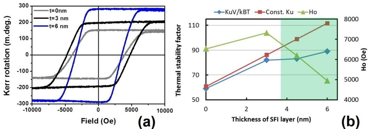
Figure 3: (a) MOKE hysteresis loop of the samples with different SFI layer thickness. (b) Estimated values of anisotropy field ( $H_o$ ) and the thermal stability factor ( $K_u V/k_B T$ ) (from dynamic coercivity), as a function of SFI layer thickness. Variation of thermal stability with SFI layer thickness for a constant  $K_u$  value of  $7 \times 10^6$  erg/cc is also shown.
