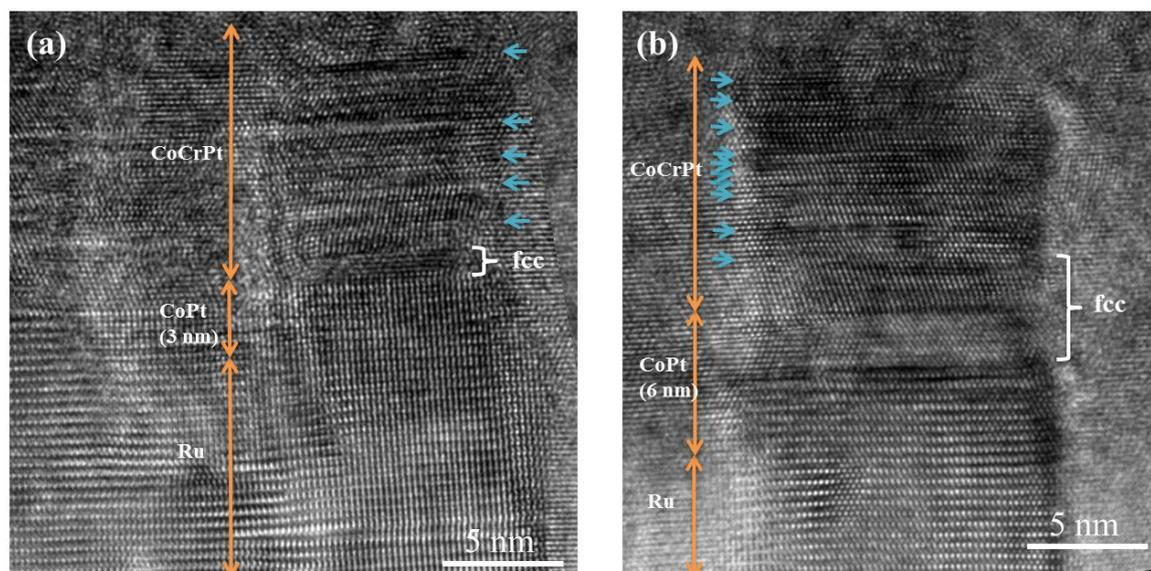
Figure 6. Typical cross-section TEM images of SFI-CoPt(*t* nm)/CoCrPt:Oxide (10 nm) samples with (a) 3 nm SFI layer and (b) 6 nm SFI layer.
