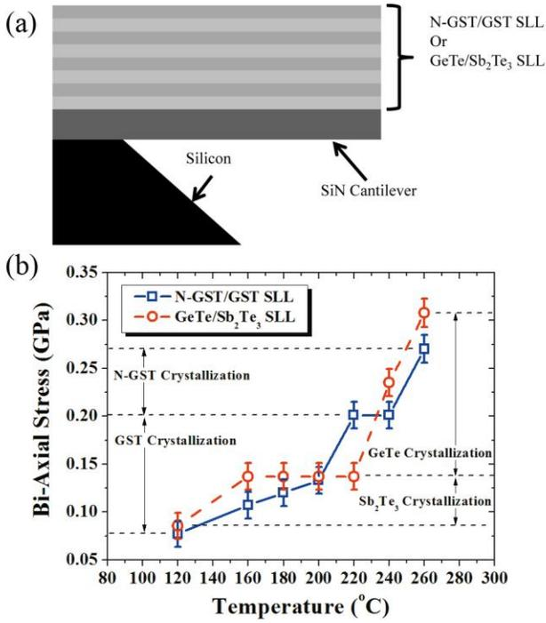
FIG. 4. (a) Cross-section of the SLL structure on the SiN cantilever and (b) Bi-axial stress of the two SLL structures annealed at different temperatures. The bi-axial stress was estimated using the bi-axial modulus of GST.
