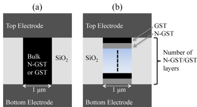
FIG. 1. Schematic cross-section of (a) N-GST and GST PCRAM and (b) N-GST/GST SLL PCRAM. Both devices have a 1  $\mu\text{m}$  diameter contact area. The total thickness of the N-GST/GST SLL and the bulk phase change materials are kept at 50 nm. The number of layers of N-GST and GST in N-GST/GST SLL were varied and their thickness changed correspondingly to make up a total thickness of 50 nm.
