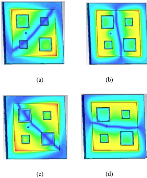
Fig. 2. Current density distribution on patch radiator at 1.578 GHz.
