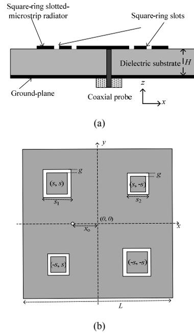
Fig. 1. Proposed antenna geometry: (a) cross-sectional view and (b) square-ring-shaped slotted-microstrip radiator.
