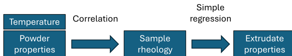
Figure 9 Illustration of the hypothesised relationship between powder properties, sample rheology and extrudate properties.
