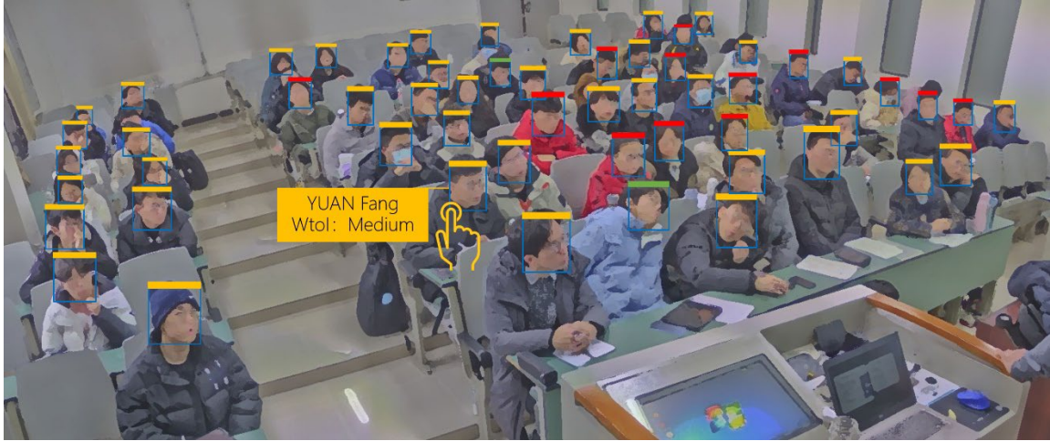
Figure 2: A showcase of NaMemo2 UI a teacher used in a class. The boxes locate the recognized student faces. The bar colors on top of the boxes show student willingness to interact (WtoI). Green means high, yellow means moderate, and red indicates low willingness. The student’s name with WtoI will appear when the box surrounding their face is clicked. The image is obscured and an alias is used to protect student privacy, and the original Chinese text in the UI is replaced with English for demonstration.
