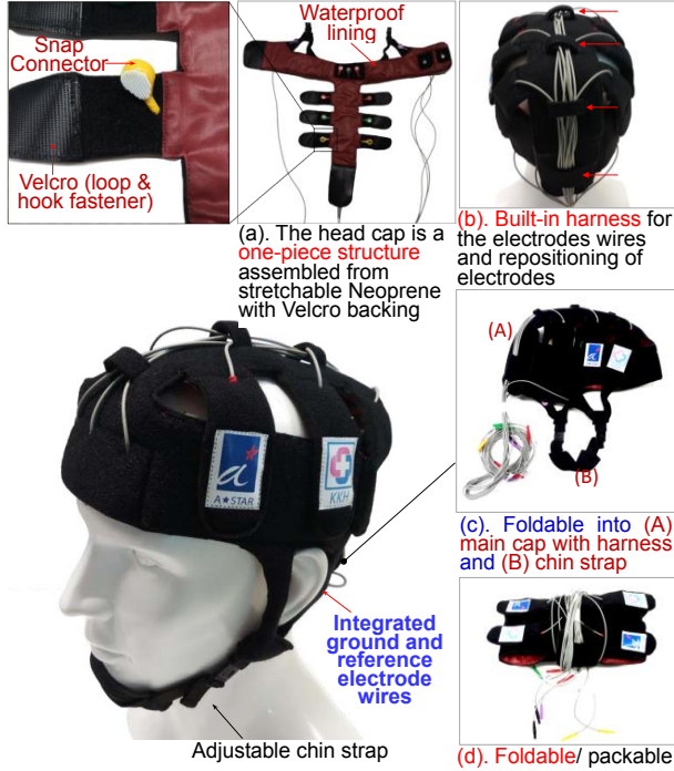
Figure 4: Photo of the fabricated dry EEG head cap integrated with EEG electrode wires as well as ground and reference electrode wires. It could be disassembled into one-piece component only. The cap is suitable for children’s head sizes of 46-52 cm and up to 60 cm for adults. The built-in harness allows for repositioning of electrodes and for adding or replacing of electrode wires while maintaining to 10-20 system for placement of electrodes on the cap.
