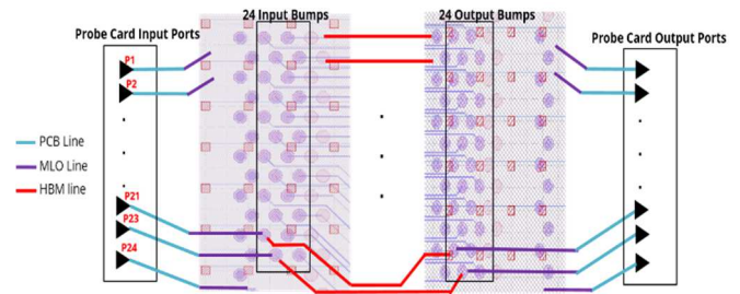
Fig. 2. Interconnect of probe card PCB, MLO and HBM lines
