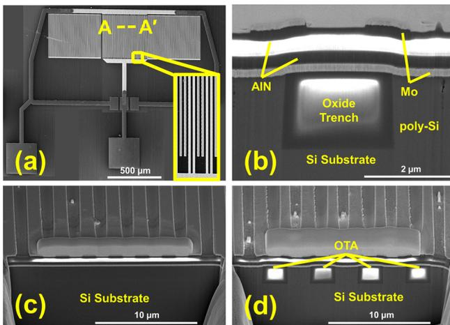
FIG. 3. SEM images of fabricated devices. (a) Top view of a device, with a close-up view of the IDT included as an inset; (b) Cross-section A–A', illustrating one oxide trench; (c) Cross-section A–A' of the device without OTA; (d) Cross-section A–A' of the device with OTA. The materials are labeled on the images.
