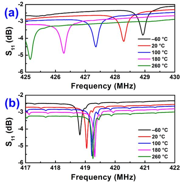
FIG. 4. Device  $S_{11}$  measurements over various operating temperatures, for devices (a) without OTA and (b) with OTA.
