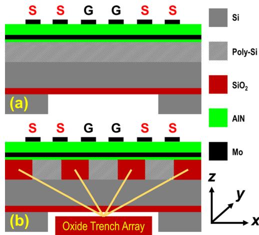
FIG. 1. Illustration of designed devices. (a) Cross-section of the AlN-on-Si resonator without OTA, as the reference design. (b) Cross-section of the designed device with OTA.
