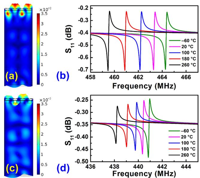
FIG. 2. Results of FEM simulation: (a) Quasi-SAW mode shape supported by the device without OTA; (b) shift in the  $S_{11}$  spectrum of the mode in (a) over a range of temperatures; (c) quasi-SAW mode shape supported by the device with OTA; and (d) shift in the  $S_{11}$  spectrum of the mode in (c) over a range of temperatures.
