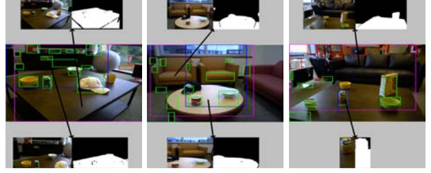
Fig. 5: Depth based filtering of 2D object proposals (best viewed in color). We only display a handful of object proposals for clarity purposes. In the soft filtering process, the blue and magenta bounding boxes are detected to contain background and undergo depth based background suppression while the red and green bounding boxes are detected to contain no major background. After the background masking process, we check the actual size of each bounding box using depth information. The red and magenta bounding boxes are identified as areas that are either too small or too big in size or do not contain depth information (holes in depth image). These 2D object proposals are discarded. The blue regions, after background suppression, and green regions are detected to potentially contain good information and are accepted as valid object proposals.
