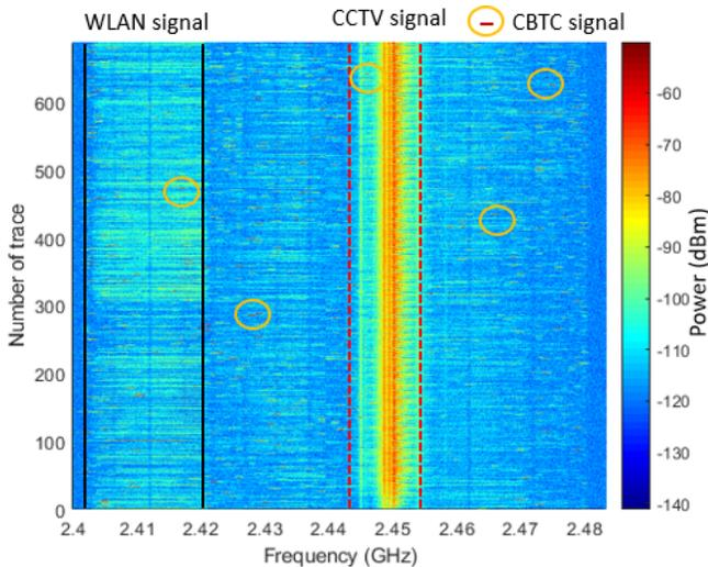
Fig. 2: Typical waterfall diagram for spectrum survey.
