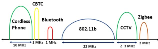
Fig. 1: Devices using 2.4 GHz ISM band in a MRT station.
