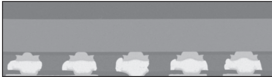
Figure 13: Post thermocompression cross sectional picture for 2 x 1.8mm top dies on bottom wafers with SOP.
