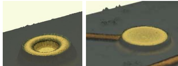
Fig 10b: RHS: Improved UBM plating with lower dishing
