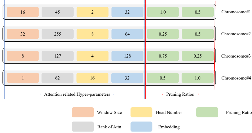
Figure 7: Visualization of the example chromosomes sampling from the gene encoding space, where the target model is a two-layer transformer. Each unit is drawn by different colors, and plays different role in the transformer model.
