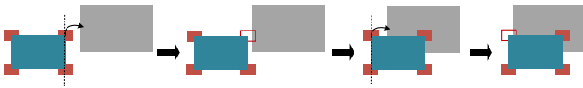
Fig. 4. Obstacle size determines whether the feet need to step on the obstacle. For long obstacles, better to step on to increase movement stability.
