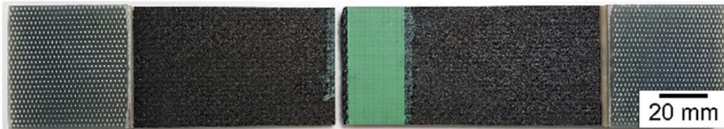
(b) 2D SVC repair
