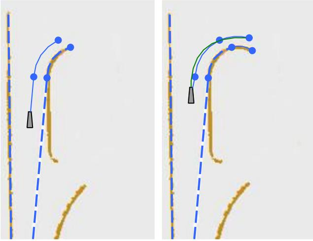
Fig. 5: An example of lane fitting and prediction, where blue point is V-point, blue dashed line is piecewise lane marking (marker & curb) fitting, blue solid line is piecewise lane prediction, and green solid line is the real-time path smoothing.
