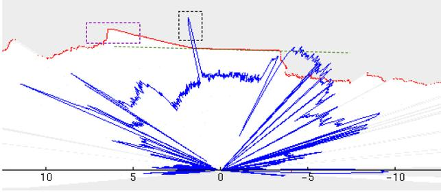
(b) Green dashed line is the laser section line on the flat road for laser's pose calibration, purple dashed box contains the interesting area for road curb, and black dashed box contains the interesting areas for lane marker.
