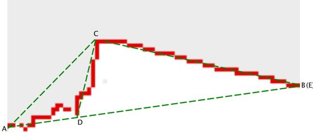
(c) 2D Convex angle for curb detection.
