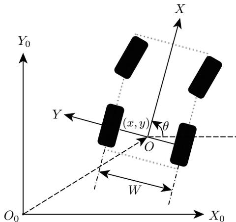
Fig. 2: Axes of odometry and vehicle.  $X_0-O_0-Y_0$  is the axis of odometry,  $X-O-Y$  is the axis of vehicle,  $(x, y)$  is the position of vehicle,  $\theta$  is the orientation of vehicle, and  $W$  is the width between left and right rear wheels.
