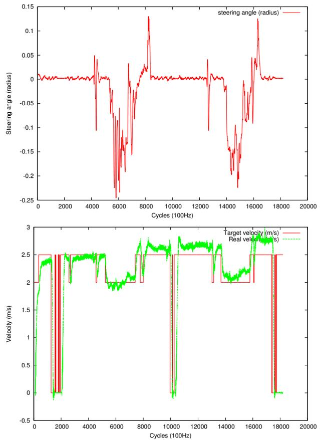
Fig. 8: The outputs of steering angle and target velocity from the LQR controller, and the real velocity from the vehicle.
