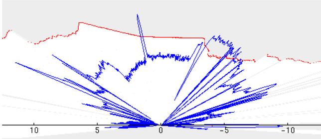
(a) 2D laser's raw data in laser's coordinate. Red curves represent the depth data and the blue curves represent the intensity data.
