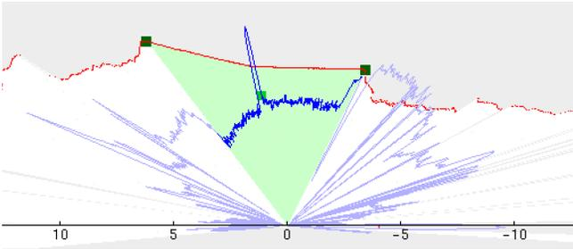
(d) Two lanes are detected from the raw data. Green point is the detected lane marker, dark green points are detected curbs, and the light green area is the road range.
