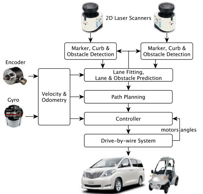
Fig. 3: System architecture for the map free 2D laser scanner based autonomous service vehicle.
