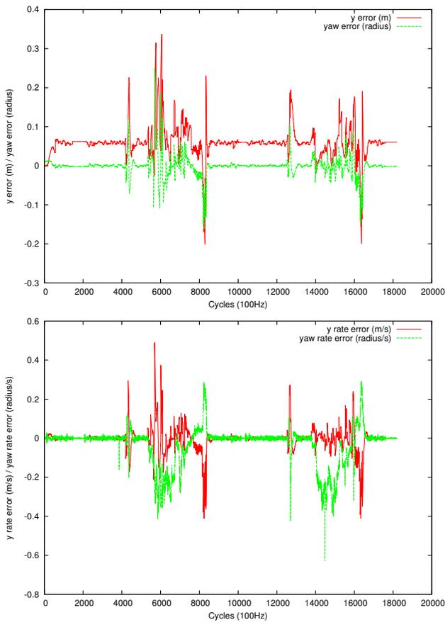
Fig. 7: Errors of  $y, \dot{y}, \theta, \dot{\theta}$  between odometry and planned path for LQR controller.
