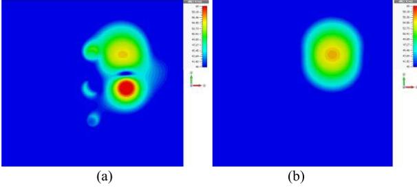
Fig. 5. Simulated  $E$ -field magnitude distribution along the  $xy$  plane at 2.44 GHz (excited by Ant. 1,  $z = 13.67$  mm). (a) With mushroom. (b) Without mushroom.
