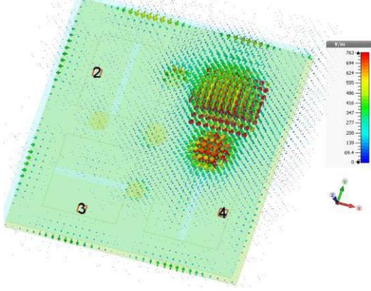
Fig. 6. 3-D  $E$ -field distribution of the proposed four-element antenna system with mushroom at 2.44 GHz (excited by Ant. 1).
