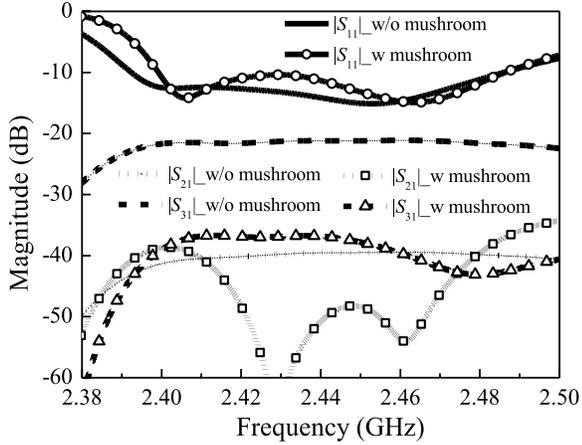
Fig. 8. Comparison of the simulated  $S$ -parameters of the four-element antenna system with/without mushroom.
