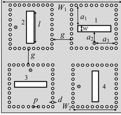
Fig. 1. Geometry of the four-element SICBS antennas.  $W_1 = 150$  mm,  $a_1 = 22.25$  mm,  $a_2 = 17.03$  mm,  $a_3 = 24.73$  mm,  $W_2 = 49.46$  mm,  $l = 48.3$  mm,  $w = 4.5$  mm,  $d = 0.5$  mm,  $p = 0.76$  mm, and  $h_1 = 1.524$  mm.
