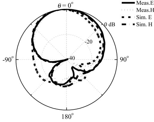
Fig. 12. Measured and simulated radiation patterns (2.44 GHz).
