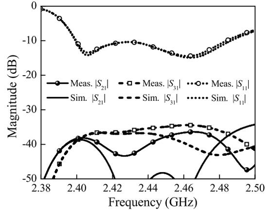
Fig. 11. Measured  $S$ -parameters of the four-element SICBS antenna system with mushroom.
