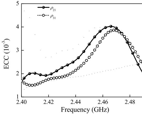
Fig. 13. Calculated ECC of the four-element antenna system.
