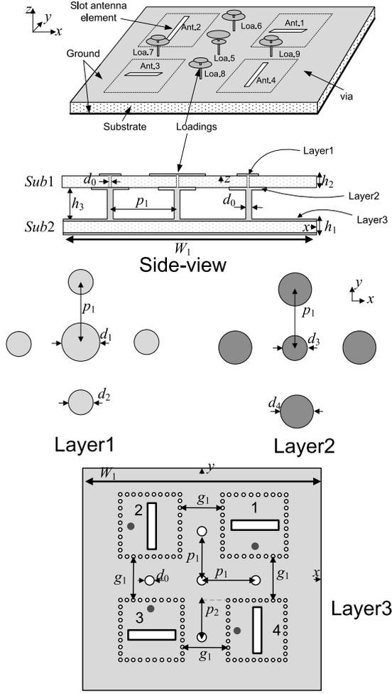
Fig. 3. Geometry of the four-element SICBS antenna system with mushroom loadings.
