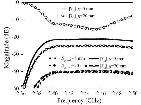
Fig. 2. Mutual coupling of the four-element SICBS antennas with the variation of  $g$ .
