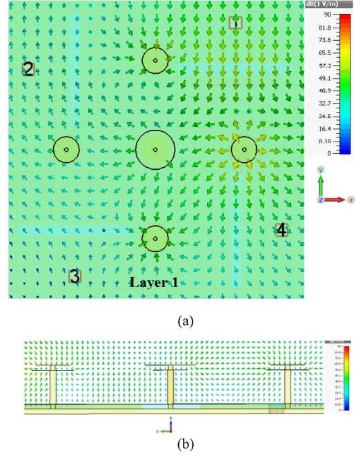
Fig. 4. Simulated  $E$ -field distribution at 2.44 GHz. (a) Layer 1 ( $xy$  plane,  $z = 13.67$  mm). (b) Cross-sectional view ( $xz$  plane,  $y = 0$  mm) (excited by Ant. 1).
