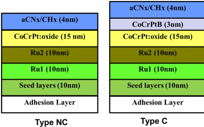
Figure 1: Sketches of the recording media structures with approximate layer thicknesses.
