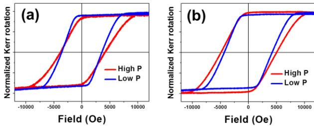
Figure 3: MOKE hysteresis loops of the (a) Type NC and (b) Type C samples fabricated by depositing the second ruthenium and recording layers at a relatively lower pressure (Low P) and higher pressure (high P) conditions.
