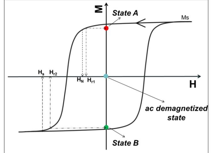
Figure 2: Schematic presentation of the three magnetic states at which MFM cluster size measurements were carried out.
