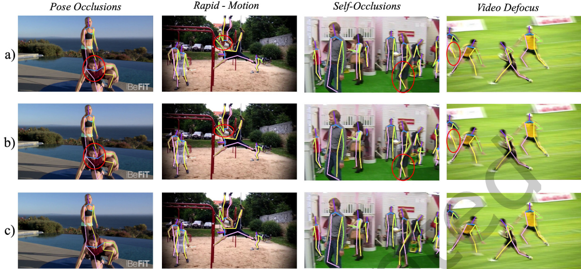
Fig. 5. Visual comparisons of c) our GLPose method against a) HRNet-W48 [40] and b) PoseWarper [4] on the challenging dynamic environments. Each column from left to right denotes the Pose Occlusions, Rapid-Motion, Self-Occlusions, and Video Defocus. Inaccurate results are highlighted with the red solid circles.
