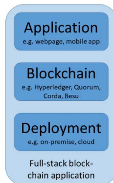
Figure 17 Layer stack of a full-stack blockchain application.
