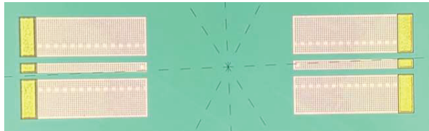
Fig. 8. Photographs of the fabricated front-back-front interconnection on the RF SOI wafer.
