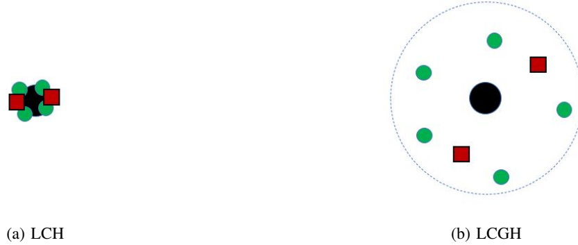
Fig. 2: The categorical cross-entropy loss in LCH encourages the hash codes to approach its class exemplar and minimize within-class variance. Conversely in LCGH, if the categorical cross-entropy loss is less than \epsilon , the loss gradient is ignored allowing within-class-variance to be retained. In the context of the example used in Fig 1, LCH encourages the hash codes of all apples to cluster around the ‘red’ exemplar while the hash codes trained by LCGH retains variance pertaining to their shade of red. The hash codes of the unseen classes, denoted by red squares, can be distinguished in LCGH but not LCH.
