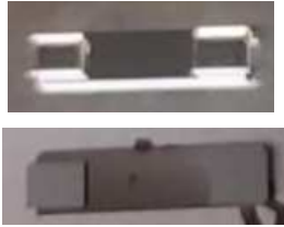
Figure 3: Bonded Glass/Die on PSPI Coated Substrate
