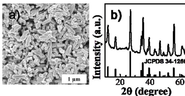
**Figure 1.** a) XRD pattern and b) SEM image of the prepared  $\beta$ -FeOOH
