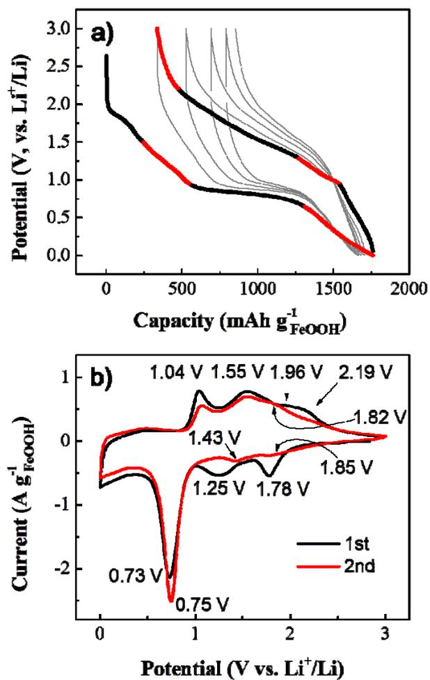
**Figure 2.** a) First five discharge/charge curve of the  $\beta$ -FeOOH at a current density of  $0.2 \text{ A g}^{-1}$ . Electrode components: 70 wt%  $\beta$ -FeOOH-1 / 15 wt% SP / 15 wt% CMC. Two colors (black and red) are used to show different regions in the first cycle; b) CV curves of the  $\beta$ -FeOOH. Scanning rate:  $0.2 \text{ mV s}^{-1}$
