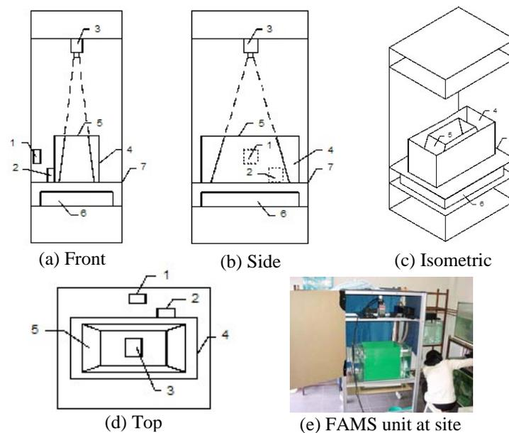
**Figure 1. The proposed fish activity monitoring apparatus. It houses fish tank, cameras and other necessary components that gives constant light and controlled test environment. (Legends: 1 - front camera, 2 - speaker, 3 - top camera, 4 - fish tank, 5 -partition, 6 - light box)**
