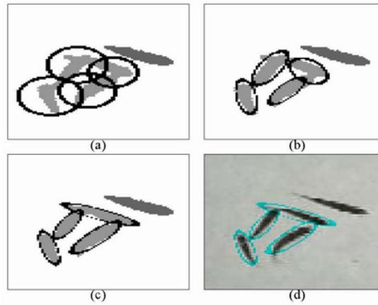
**Figure 4. Steps taken in blob splitting process. (a) Clustering based on Euclidean distance that gives round-shape fitting; (b) Improved fitting by computing Mahalanobis distance and computing ellipse parameters  $\{\gamma_i^t\}$ ; (c) Parameters of ellipses  $\{\gamma_i^t\}$  are perturbed to give better fitting; (d) Final result of the blob**
