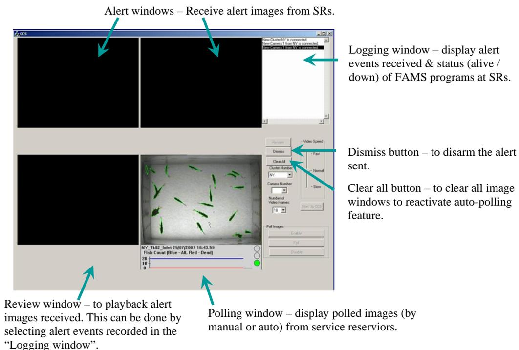
**Figure 6. User interface of FAMS network software that runs at the control centre.**
