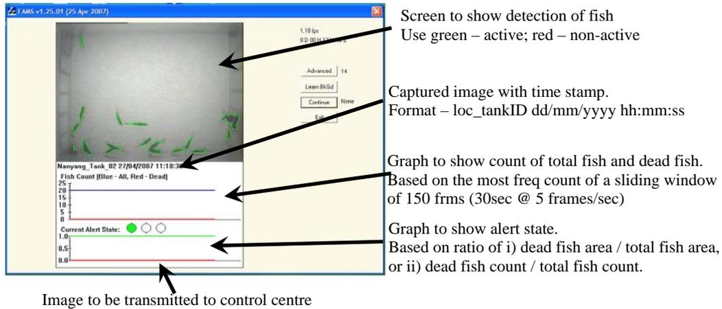
**Figure 7. User interface of FAMS unit that runs at service reservoir.**
