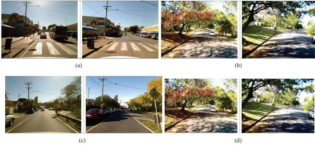
Fig. 3. Examples which can be recognized with a CNN model but can not be recognized using traditional BoW+HV solution due to varied lighting conditions.
