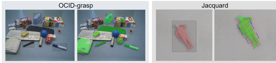
Fig. 2. Example predictions on the OCID-grasp and Jacquard dataset. Left of each pair: original images and box prompts for desired object to grasp. Right of each pair: Top-3 grasps and instance masks predicted by the model.
