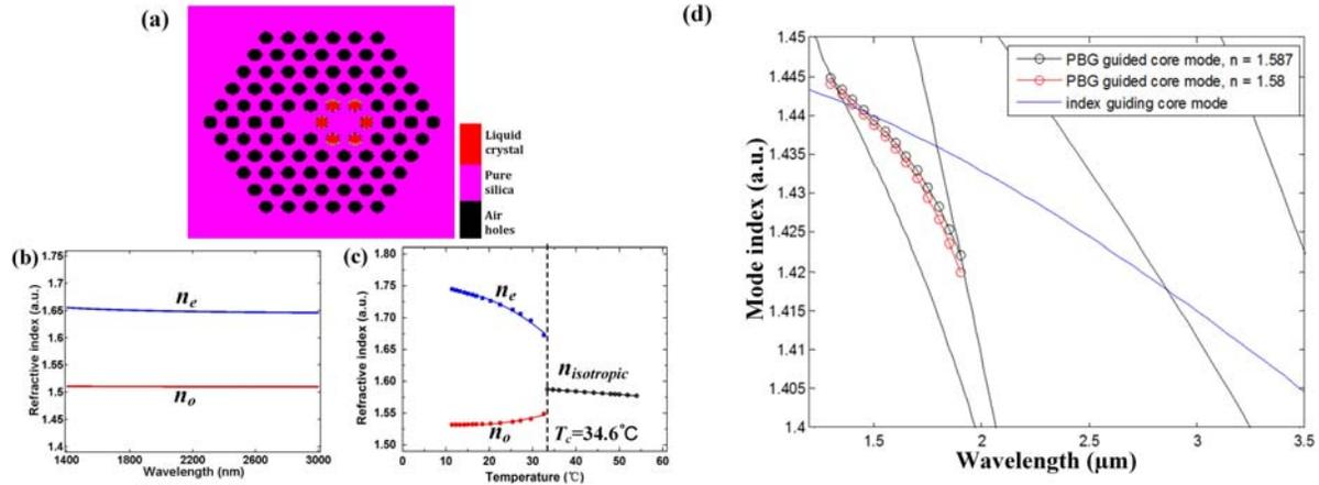
Fig. 1. (a) Refractive index (RI) profile of the liquid crystal filled twin core PCF; (b) Dispersion curve of 5CB; (c) Temperature dependence of RI of 5CB; (d) Mode dispersion curves of the two cores in the hybrid PCF.
