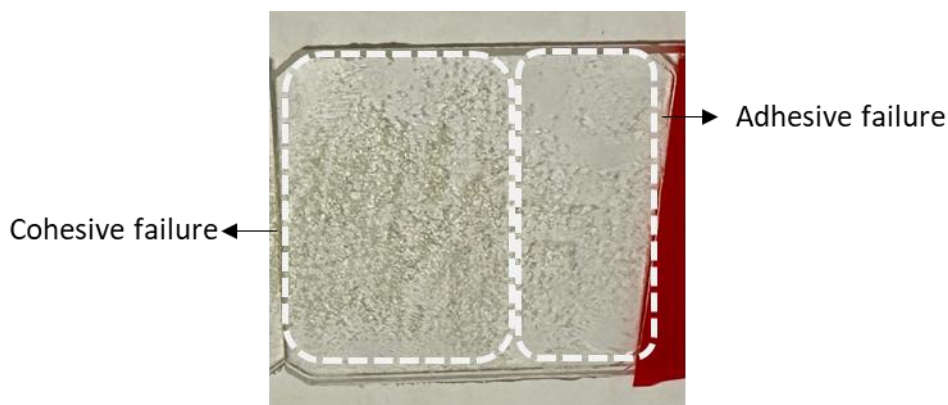
Figure S8. Glass substrate after UV irradiation ( \lambda_{\text{max}} = 340 \text{ nm} , I = 10 \text{ mW cm}^{-2} ), showing cohesive and adhesive failure.
