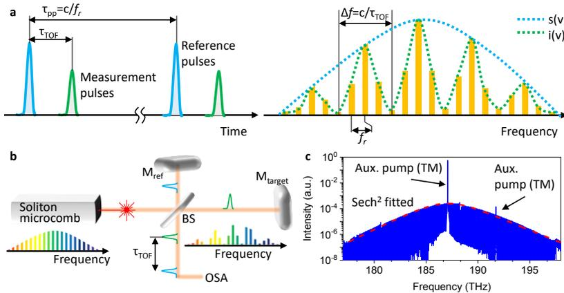
**Figure 1. (a)** Principle of spectral resolved interferometer for distance measurement **(b)** Experimental set up of soliton microcomb based spectral interferometer for precise distance measurement. Inset is an example spectrum of soliton microcomb used in this study.  $M_{ref}$ : reference mirror,  $M_{target}$ : target mirror, and BS: beam splitter, OSA: optical spectrum analyzer. **(c)** Optical spectrum of single soliton microcomb.
