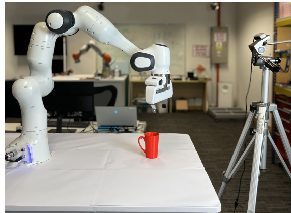
Fig. 1: An illustration of a single-camera visual policy setup for robot manipulation tasks, with a front-facing third-person camera.
