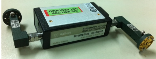
Fig. 1. Travelling standard for attenuation in WR-15 waveguide band.
