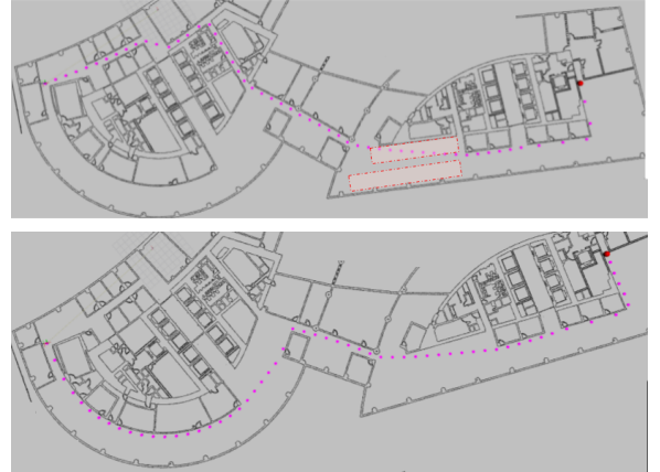
Fig. 5. Two test routes. route 1: indicated by pink dots on the top image; route 2: indicated by pink dots on the bottom image. The most difficult areas are marked as dashed rectangles. The cubicles are missing from both sides of the real path.
