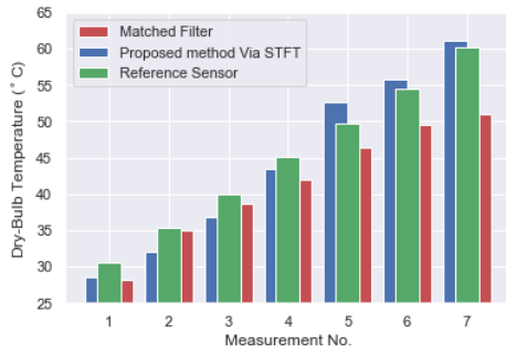
Fig. 4. Actual vs estimated dry-bulb temperatures using the proposed signal processing algorithm and the matched filter approach.
