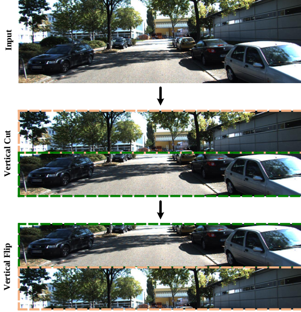
Fig. 3. Illustration of the CutFlip technique. The CutFlip contains two key steps: vertical cut and vertical flip.
