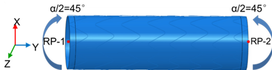
Figure 3. Bending test: boundary conditions and loads [19].
