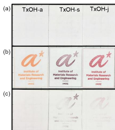
Figure 5. Paper probes (2.5 x 5.0 cm) inkjet-printed with TxOH-a , TxOH-s and TxOH-j before (a) and after exposure to TFA fumes (b), as well as 1 hour on standing in ambient laboratory humidity after exposure to TFA fumes (c).
