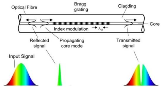
Fig. 1: Schematic of a grating structure [8]
