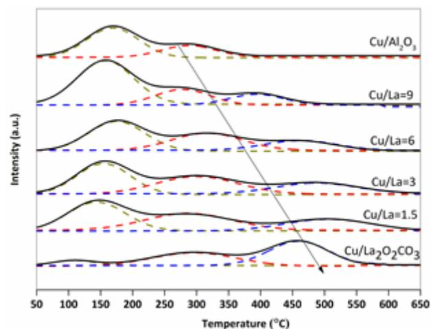
Figure 3.  $\text{CO}_2$ -TPD profile of the catalysts.
