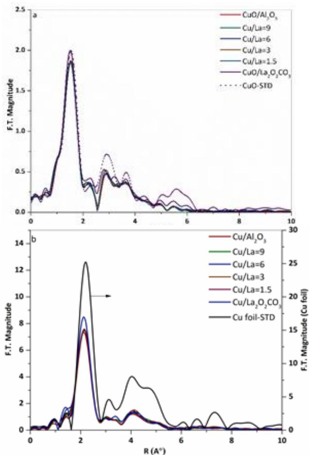
Figure 6. Cu K-edge EXAFS spectra of a) CuO/ La<sub>2</sub>O<sub>2</sub>CO<sub>3</sub>-Al<sub>2</sub>O<sub>3</sub> with different ratio of Cu/La, and CuO/ La<sub>2</sub>O<sub>2</sub>CO<sub>3</sub>, b) Cu/ La<sub>2</sub>O<sub>2</sub>CO<sub>3</sub>-Al<sub>2</sub>O<sub>3</sub> with different ratio of Cu/La, and Cu/ La<sub>2</sub>O<sub>2</sub>CO<sub>3</sub>.
