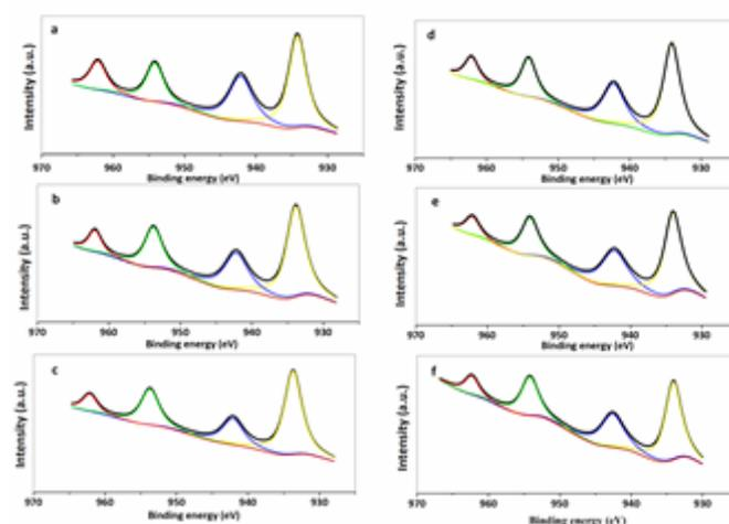
Figure 5. Copper 2p core level XPS spectra of the calcined catalysts, a) Cu/Al<sub>2</sub>O<sub>3</sub>, b) Cu/La=9, c) Cu/La=6, d) Cu/La=3, e) Cu/La=1.5, f) Cu/ La<sub>2</sub>O<sub>2</sub>CO<sub>3</sub>.
