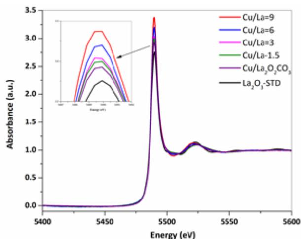
Figure 7. XANES spectra of the reduced Cu-La<sub>2</sub>O<sub>2</sub>CO<sub>3</sub>/Al<sub>2</sub>O<sub>3</sub> with different Cu/La ratios and Cu/ La<sub>2</sub>O<sub>2</sub>CO<sub>3</sub> at the La L<sub>III</sub>-edge.
