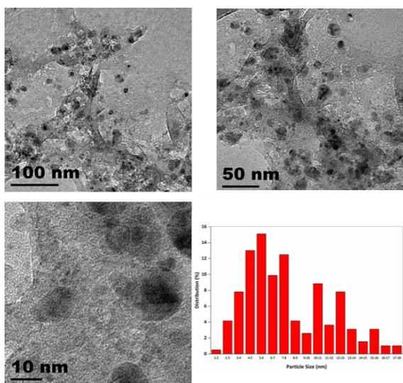
Figure 2. TEM images and particle size distribution of  $\text{Cu-La}_2\text{O}_2\text{CO}_3/\text{Al}_2\text{O}_3$  sample with a Cu/La ratio=6.
