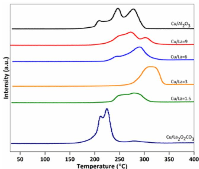
Figure 4. TPR profiles of the catalysts.
