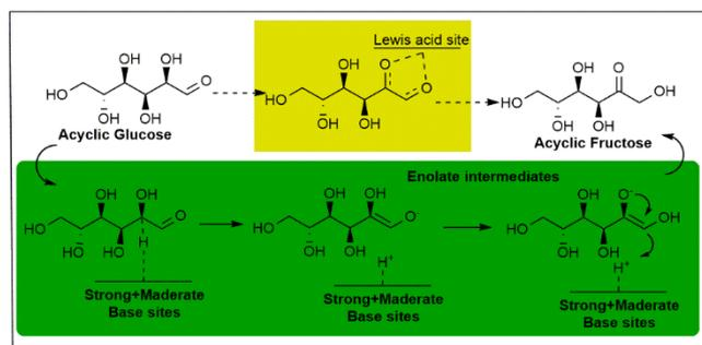
Figure 9. Proposed reaction mechanism adapted from previous reports<sup>9, 38, 39</sup> for glucose isomerisation to fructose over the synthesized catalysts.
