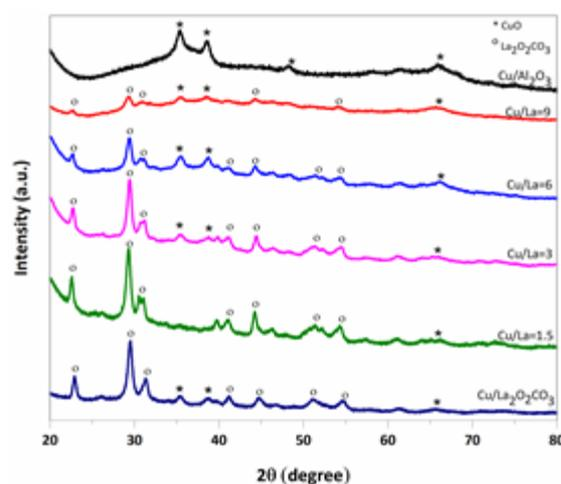
Figure 1. XRD spectra of the calcined catalysts.
