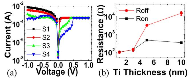
Fig. 3. (a) Typical resistive switching characteristics of all samples, showing no switching phenomena in S1 & S2 and good switching behaviors in S3 & S4. (b) On/off resistance plot of all samples versus Ti capping layer thickness.
