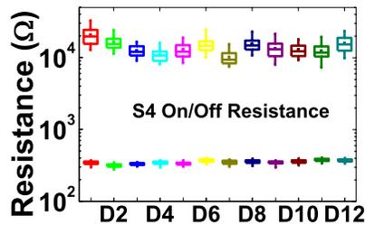
Fig. 4. Device-to-device on/off resistance uniformity plot of S4. Data taken from 100 DC cycles of 12 randomly selected devices across 8 inch wafer.
