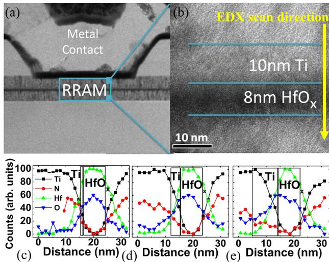
Fig. 1. (a) High resolution TEM image of S4 with 10nm Ti capping layer, confirmed the thickness of ALD HfO<sub>x</sub> deposition of 8nm. EDX line scan was performed along the direction indicated by the arrow in (b) and spatial profile was plotted for S1 (c), S3 (d) and S4 (e) with Ti capping layer thickness of 1, 5 and 10 nm, respectively.
