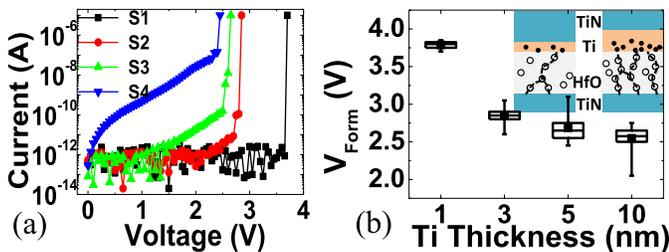
Fig. 2. (a) Initial device forming curve of all 4 samples, with forming voltage in the range of 2-4 V. (b) Forming voltage distribution box plot of 4 samples (collected from 10-20 devices each) versus Ti capping layer thickness. Larger fluctuations are observed in thick Ti capping devices. Inset schematically illustrates the origin of forming voltage fluctuations.
