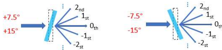
Figure S8. Measure scheme for tilting metagrating respectively at cases of \pm 7.5^\circ and \pm 15^\circ .
