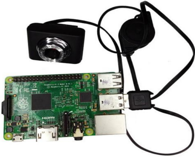
Fig. 8. An 8 MP Camera module interfaced to a Raspberry Pi board.
