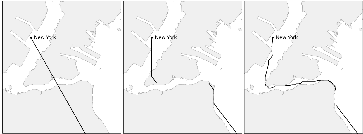
FIGURE 5: A route originating from the Port of New York, obtained using grids of varying resolutions (L12, L16, L19). Finer grids capture complex terrain features more accurately, resulting in more precise estimates of travel costs.
