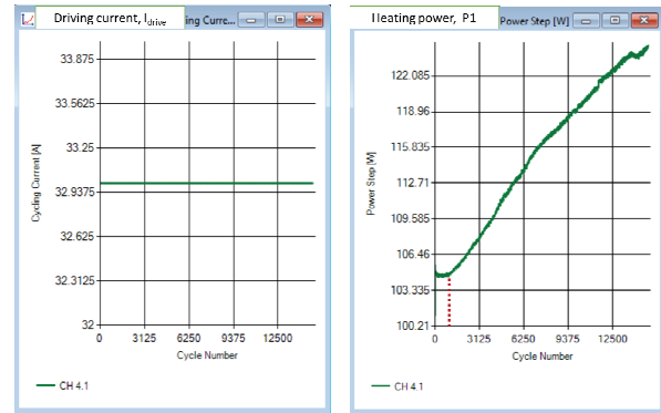
Fig. 12 Driving current and heating power apply to the test vehicle for transient thermal test the power cycling test for test vehicle 2
