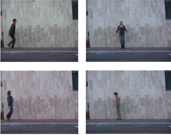
Fig. 3. Neck point detected using proposed algorithm. Neck is shown in red color in each frame.
